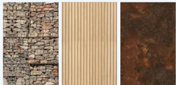
Figure 3.5 Examples of 'natural materials' — Gabion walling, timber and corten steel
